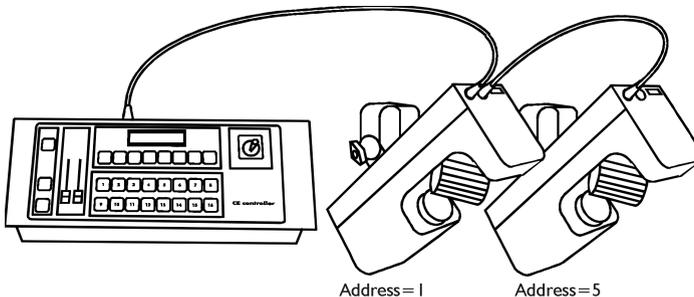
Connect your controller to the “DMX in” socket on the first unit, using a 3-pin XLR cable. If you are using a controller with a 5-pin DMX output, you will need to use a 5 to 3 pin adaptor with pins 2 and 3 swapped (pin 2 is ‘hot’). Connect the next unit, if you have one, to the DMX output plug.
