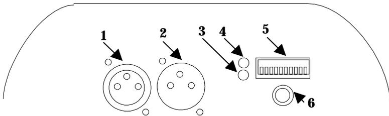
5. **Dip switches**. Dip switches 1-9 set the DMX channel that the unit will respond to (in binary code) when a DMX controller is being used. Switch 10 sets the stand alone 'group' of the unit when in stand-alone mode, either 1 (off) or 2 (on). See the last page of this booklet for help on setting the switches.
