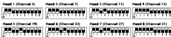
The dipswitches are set in binary code (1 = switch 1 on). To work out how you need to set the dipswitches to get a certain channel number, use the following step-by-step procedure:
